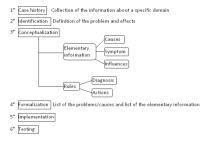
Figure 2: description of the formalization's process
